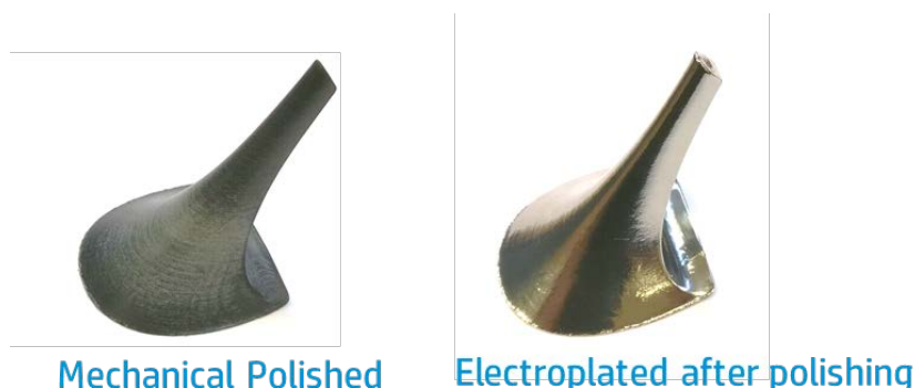
Figure 10: High heel electroplated after mechanical polishing
