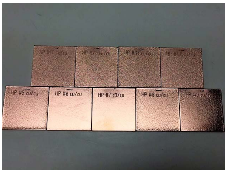
Figure 7: Preliminary results for plating with SAT Plating gas activation technology in MJF parts
