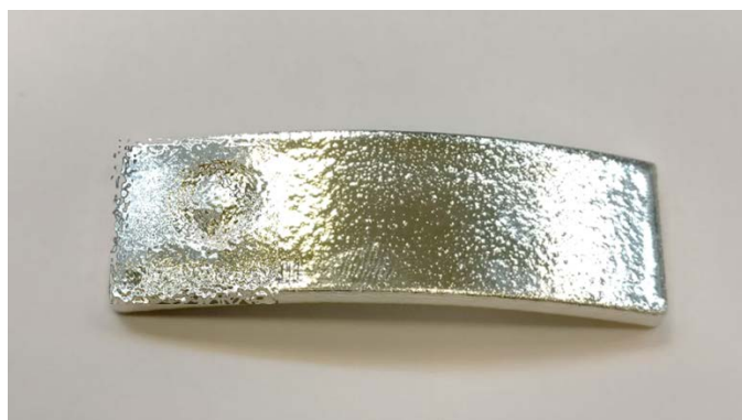
Figure 13: Raw part with decorative Jet Metal process
